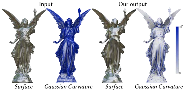
Fig. 25. Our algorithm reduces Gaussian curvature, measured per each vertex as its angle deficit divided by its 1-ring area. Model from the Stanford 3D Scanning Repository.
